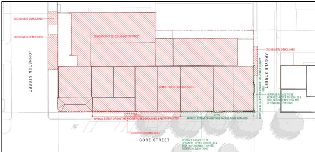
Figure 2: Extent of additional demolition shown in red Source: SJB (August 2023)
