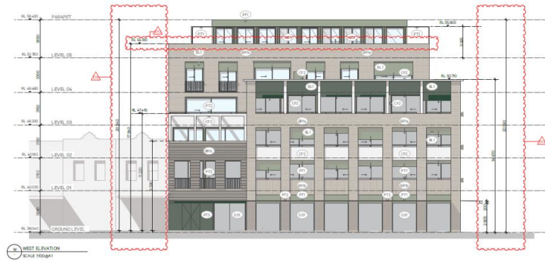
Figure 35. West (Nicholson Street) elevation of proposed infill development. (Source: Kennedy Nolan, dated 18 September 2023)
