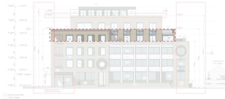
Figure 39. Marked up south (Liverpool Street) elevation showing Level 3 (outlined) which we recommend be deleted. Adapted from Kennedy Nolan drawing TP201.
