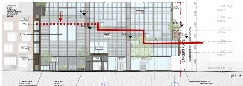
Figure 8: red dashed – preferred street wall height; solid line - proposed street wall height (Church Street)
