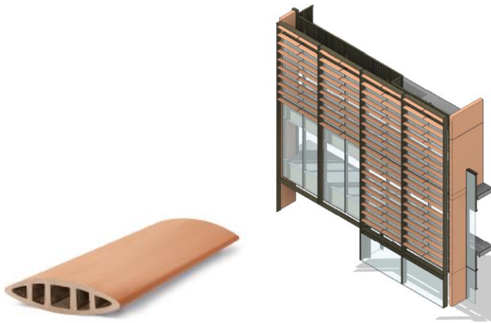
Image 9: the terracotta baguette and isometric section of the street wall façade (source: pages 42 and 43 of the Urban Context Report)
