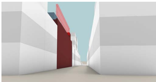
Figure 74. Slade Knitwear sign looking South, parapet of the neighbouring buildings to the south aligned with upper-level setbacks of 11m.
