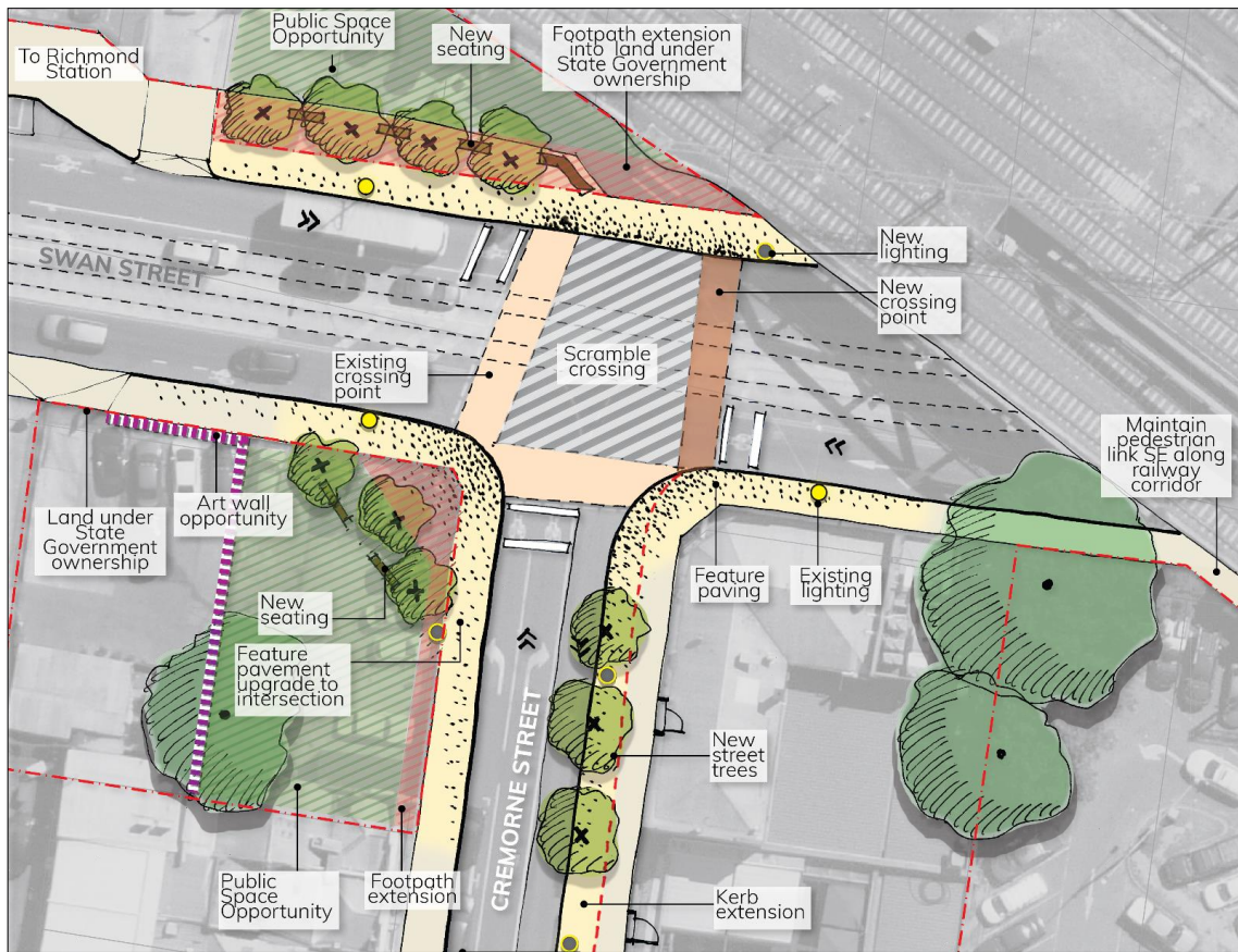
Image 10- Hotspot-Cremorne Street and Swan Street intersection
