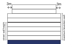
Figure 38. Diagram demonstrates the relationship between height, street wall height, boundary wall and building separation (6-8 storeys)
