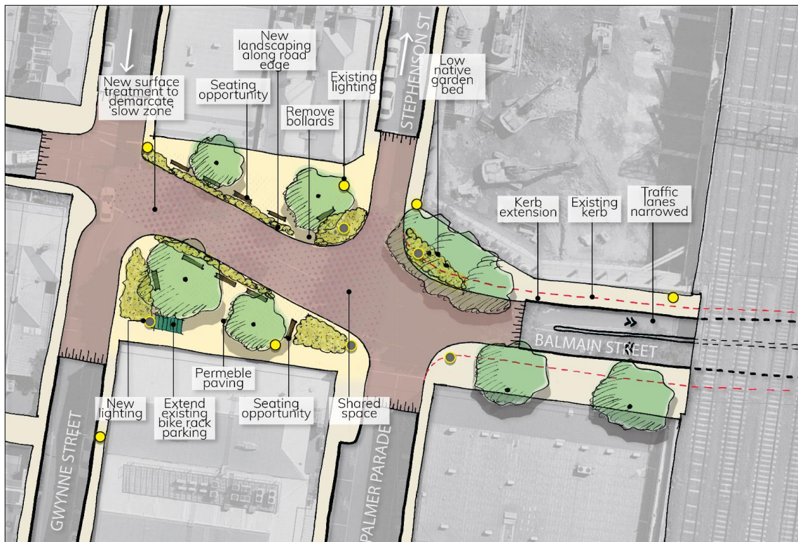
Image 11-Hotspot-Balmain Street (West of underpass)
