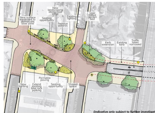
Figure 3.4 – Hotspot 4 - Balmain Street, west of the underpass
