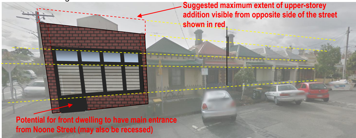
Above: Annotated image showing how the existing building and adjoining terrace should inform the proportions of a proposed new building.
