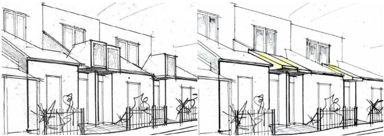
Image: Sketch plan of originally proposed (left) compared to modified (right) front entry canopies.
