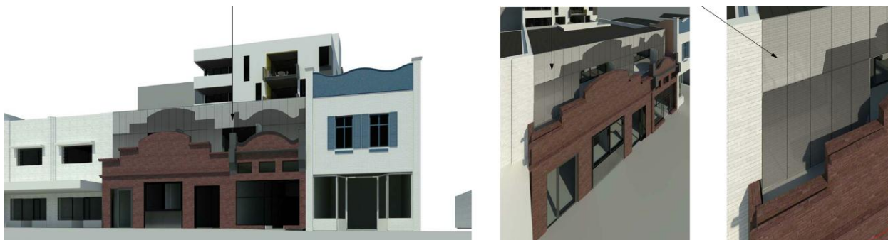
Figure 3: illustration of a silhouette of the front parapets imposed onto the screen
