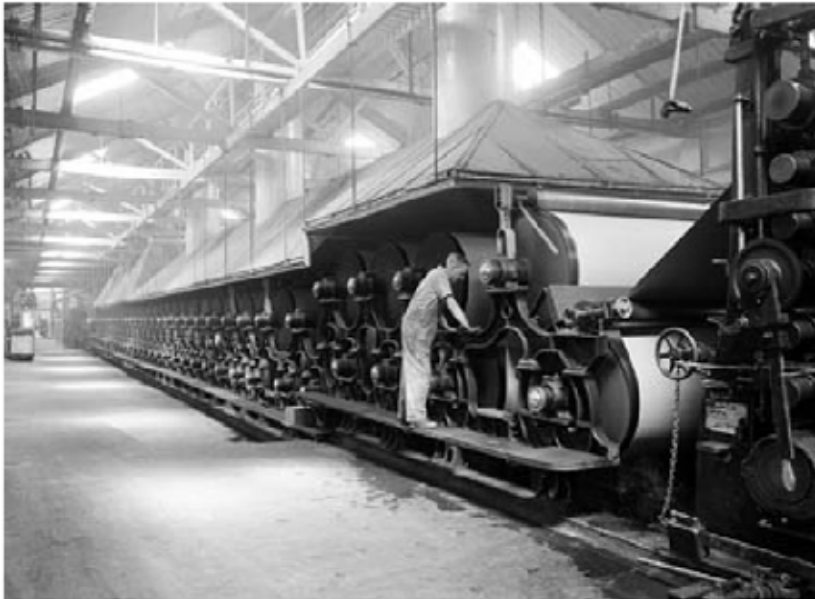
Paper making machine (probably in South Mill) c 1945, National Archives photo A1200, L2550
