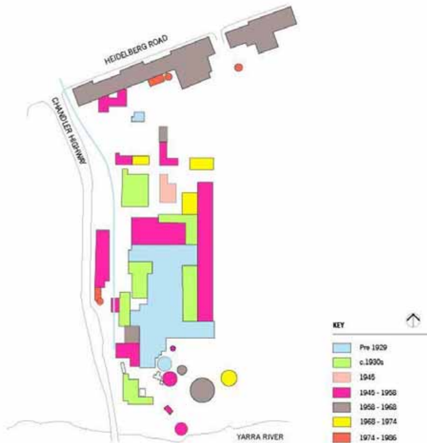
Figure 5 Indicative plan of the primary phases of development of the mill Source: Lovell Chen P/L
