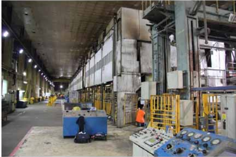
Figure 5 View looking east within F6 showing the Fourdrinier-Inverform paper making machine
