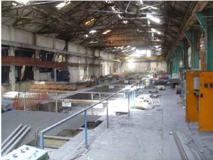
Interior of South Mill showing pits beneath former paper machines
