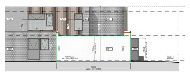
Figure 9: Proposed wall on boundary with compliant area (green) and area exceeding 3.6m (red)
