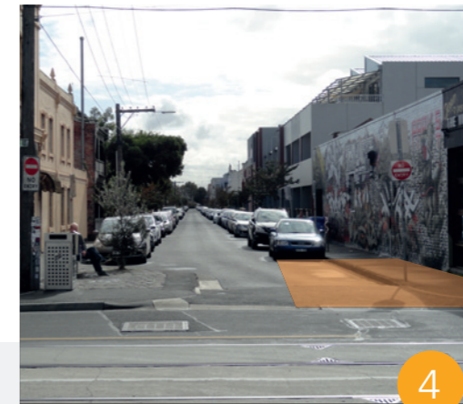
Kerb Outstand Upgrade Install a new kerb outstand to east, and repave both sides with sawn bluestone. Plant ginkgo tree.
