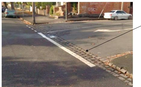
A wet crossing with a one or two pitcher wide layback. This will be built where there are no existing bluestones in the ramp or pedestrian
