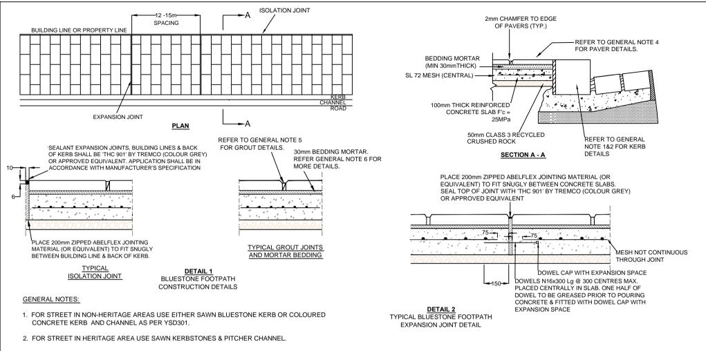
3. SAWN BLUESTONE KERBSTONES ARE 300\*300mm WITH A 25mm BULLNOSE. LENGTH IS TYPICALLY 1000mm WITH A MINIMUM LENGTH OF 800mm. STANDARD OUTSIDE RADIAL DIMENSIONS FOR CORNER STONES ARE 610mm AND 910mm.
