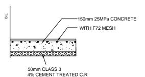
INDUSTRIAL CONCRETE FOOTPATH WITH ASPHALT SURFACE (ICAF)
