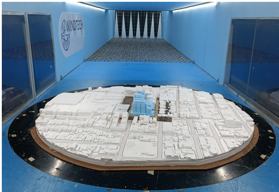
Figure 1e: Photograph of the Wind Tunnel Model (Proposed Site Conditions, view from the west)
