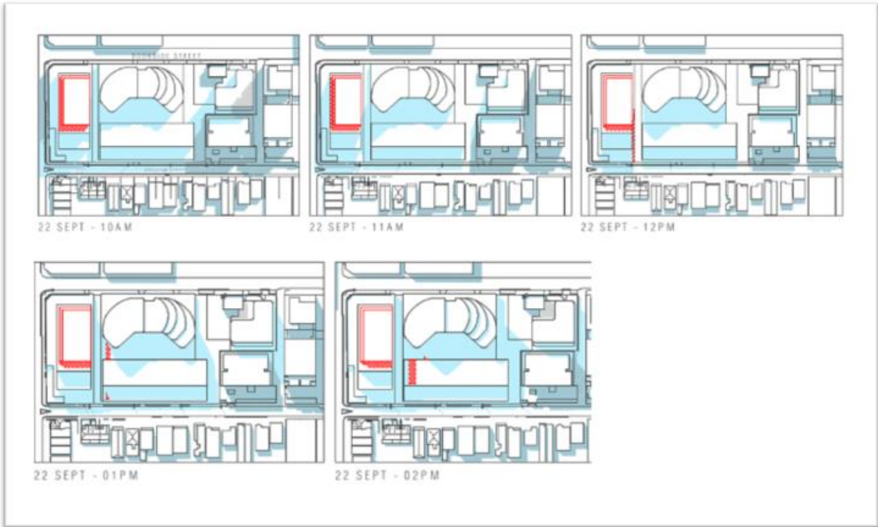
Figure 43: Additional shadows cast by two upper-most levels of Building A. Source: Applicant email 3 August 2023
