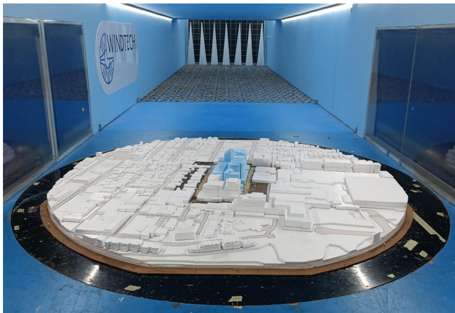
Figure 1c: Photograph of the Wind Tunnel Model (Proposed Site Conditions, view from the east)
