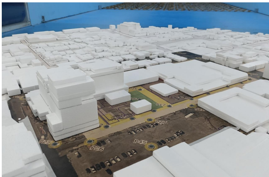
Figure 1g: Photograph of the Wind Tunnel Model (Existing Site Conditions, close-up view from the north-east)
