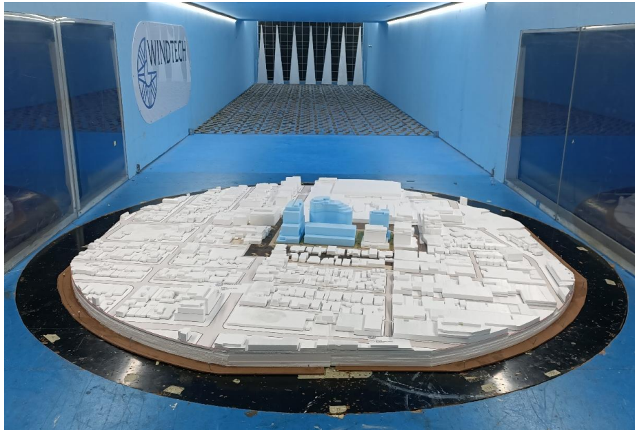
Figure 1d: Photograph of the Wind Tunnel Model (Proposed Site Conditions, view from the south)
