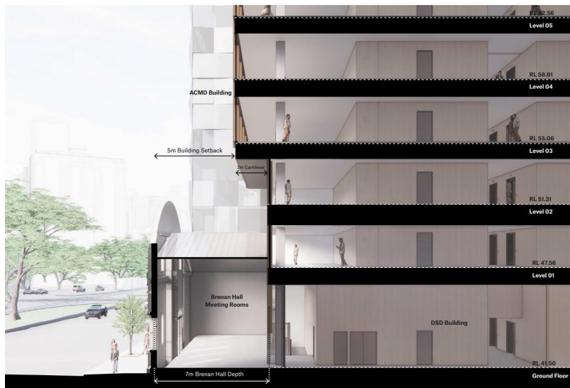
Figure 25 – Section showing cantilever of upper levels over the Brenan Hall extracted from p. 37 of the Urban Context Report and Design Response
