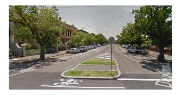
DBYD search shows there are gas lines and NBN near the kerb (service proving needed to confirm proximity to kerb)
